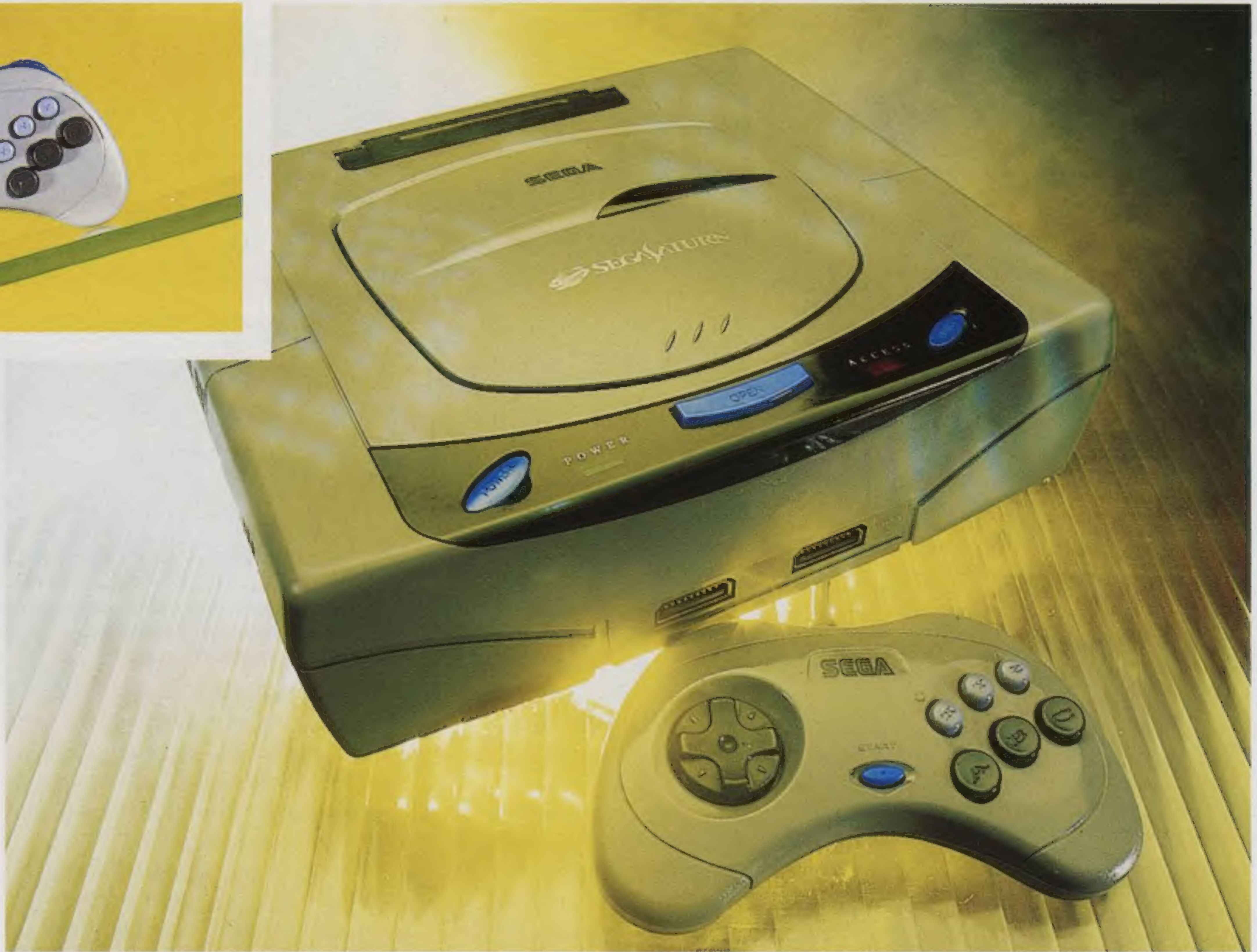
The Saturn has an all-over matt-grey finish and a rather conventional joypad (top left). Unlike the PlayStation, all the Saturn's settings are saved in SRAM using its internal battery. SRAM carts can be plugged into the cartridge slot
